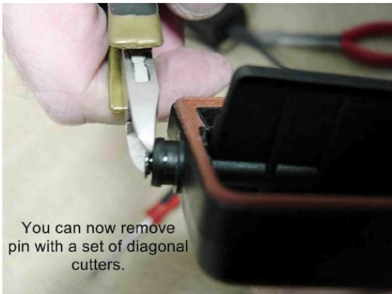
You can now remove pin with a set of diagonal cutters.
