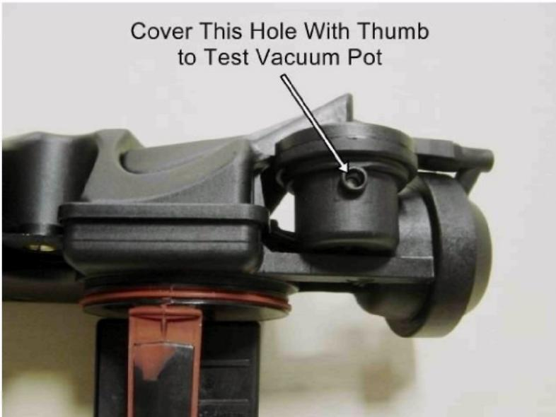
Close flapper valve all the way, then cover this hole with your thumb, then release flapper valve. Valve will spring back approx this much if pot is good. If pot is bad, flapper will open all the way when released.
